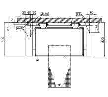
**Electric** Supply voltage: 400 V/3N ph/50/60 Hz Total Watts: 20.6 kW Installation:
